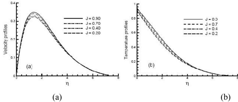
Fig. 11 (a) Velocity and (b) temperature profiles for different values of Joule heating parameter  $J$  against  $\eta$  with other fixed values  $Pr = 0.72$ ,  $M = 1.0$ .
