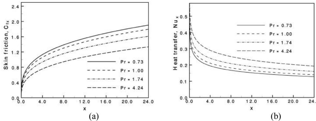
Fig. 20. (a) Variation of skin friction coefficients and (b) variation of rate of heat transfer against  $x$  for varying of  $Pr$  with  $Q = 0.01$  and  $p = 1.0$ .
