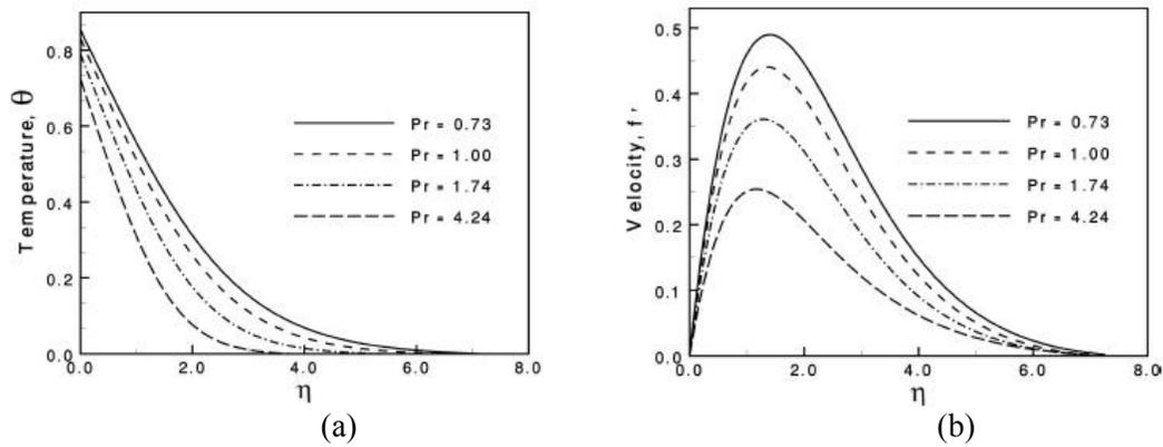
Fig. 17. (a) Variation of temperature profiles and (b) variation of velocity profiles against  $\eta$  for varying of  $Pr$  with  $Q = 0.01$  and  $p = 1.0$ .
