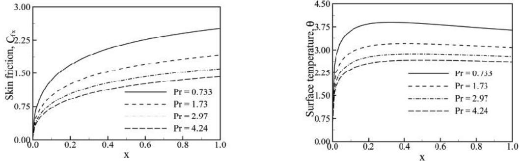
Fig. 8. (a) Variation of skin friction coefficients and (b) variation of surface temperature distributions against  $x$  for varying of  $Pr$  with  $M = 0.10$ ,  $n = 0.01$  and  $p = 0.25$ .
