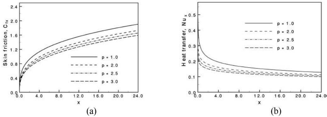
Fig. 19. (a) Variation of skin friction coefficients and (b) variation of rate of heat transfer against  $x$  for varying of  $p$  with  $Q = 0.01$  and  $p = 1.0$ .
