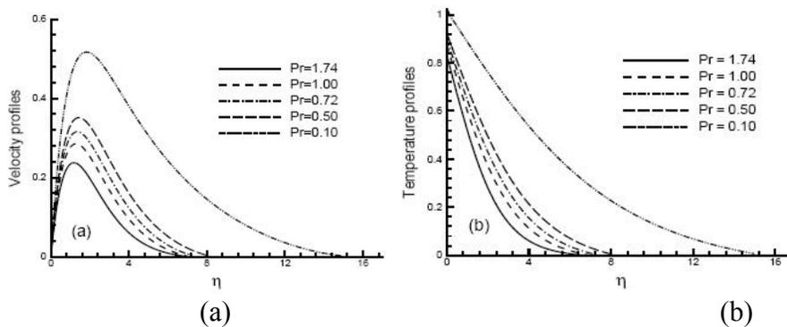
Fig. 12. (a) Velocity and (b) temperature profiles for different values of Prandtl number  $Pr$  against  $\eta$  with other fixed values  $J = 0.005$ ,  $M = 1.0$
