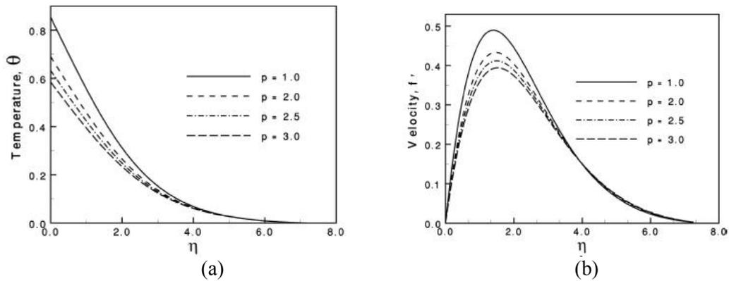
Fig. 16. (a) Variation of temperature profiles and (b) variation of velocity profiles against  $\eta$  for varying of  $p$  with  $Q = 0.01$  and  $Pr = 0.73$ .
