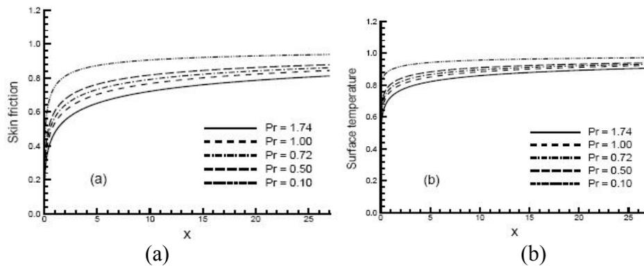
Fig. 14. (a) Skin friction and (b) surface temperature against  $x$  for different values of Prandtl number  $Pr$  with  $M = 1.0, J = 0.005$ .
