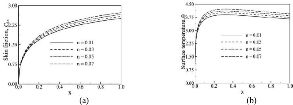
Fig. 7. (a) Variation of skin friction coefficients and (b) variation of surface temperature distributions against  $x$  for varying of  $n$  with  $M = 0.10$ ,  $Pr = 0.733$  and  $p = 0.25$ .
