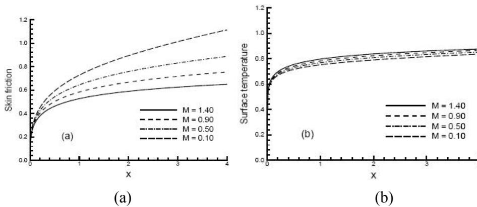
Fig. 13. (a) Skin friction and (b) surface temperature against  $x$  for different values of magnetic parameter  $M$  with fixed parameter  $Pr = 0.72, J = 0.07$ .
