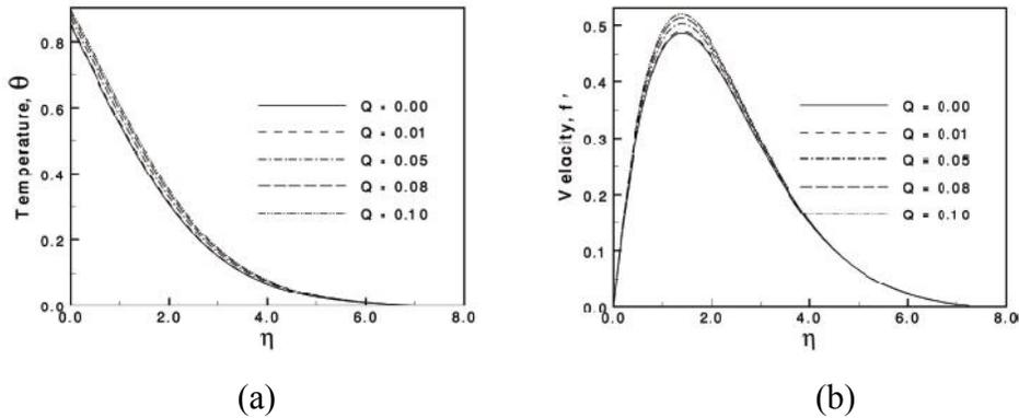
Fig. 15. (a) Variation of temperature profiles and (b) variation of velocity profiles against  $\eta$  for varying of  $Q$  with  $p = 1.0$  and  $Pr = 0.73$ .
