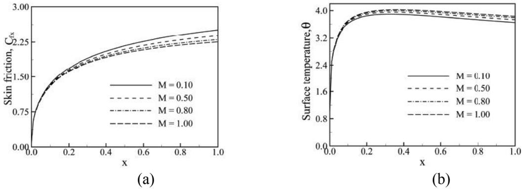
Fig. 6. (a) Variation of skin friction coefficients and (b) variation of surface temperature distributions against  $x$  for varying of  $M$  with  $n = 0.01$ ,  $Pr = 0.733$  and  $p = 0.25$ .
