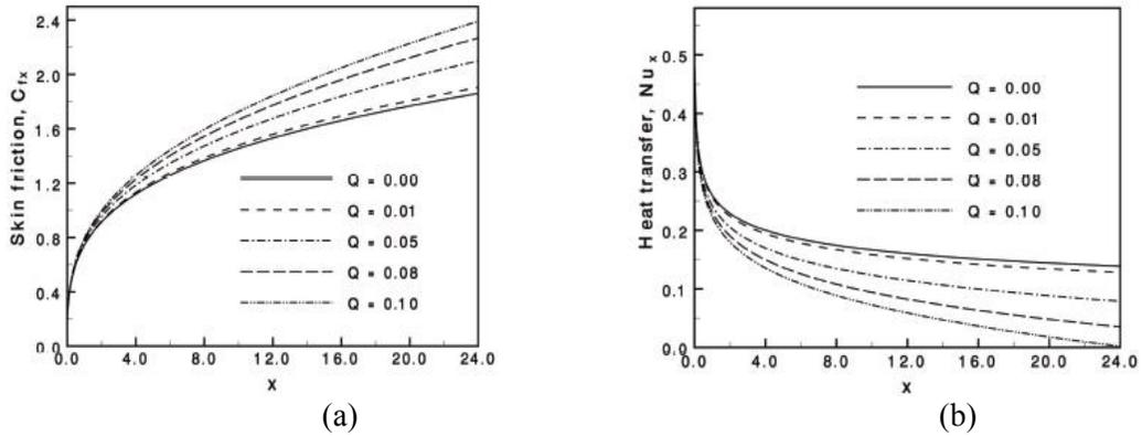
Fig. 18. (a) Variation of skin friction coefficients and (b) variation of rate of heat transfer against  $x$  for varying of  $Q$  with  $p = 1.0$  and  $Pr = 0.73$ .
