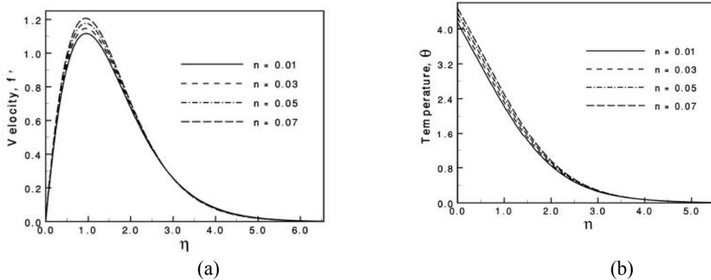
Fig. 3. (a) Variation of velocity profiles and (b) variation of temperature profiles against  $\eta$  for varying of  $n$  with  $M = 0.10$ ,  $Pr = 0.733$  and  $p = 0.25$ .
