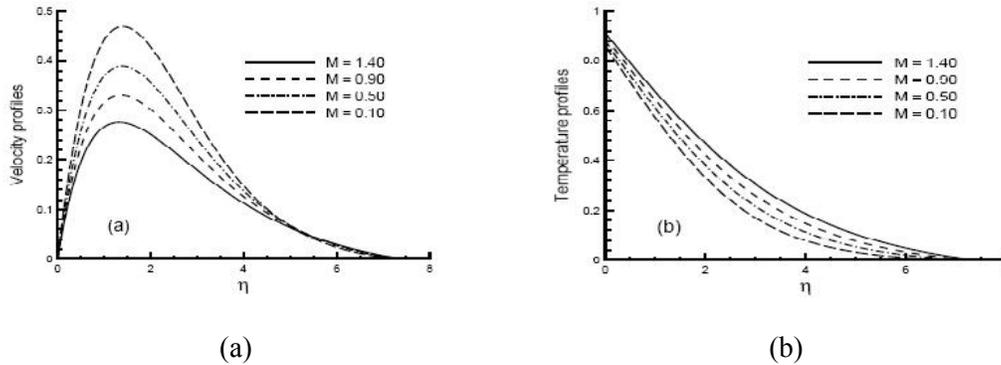
Fig. 10. (a) Velocity and (b) temperature profiles for different values of magnetic parameter  $M$  against  $\eta$  with other fixed values  $Pr = 0.72$ ,  $J = 0.07$ .
