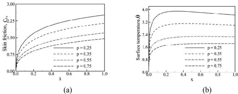
Fig. 9. (a) Variation of skin friction coefficients and (b) variation of surface temperature distributions against  $x$  for varying of  $p$  with  $M = 0.10$ ,  $n = 0.01$  and  $Pr = 0.733$
