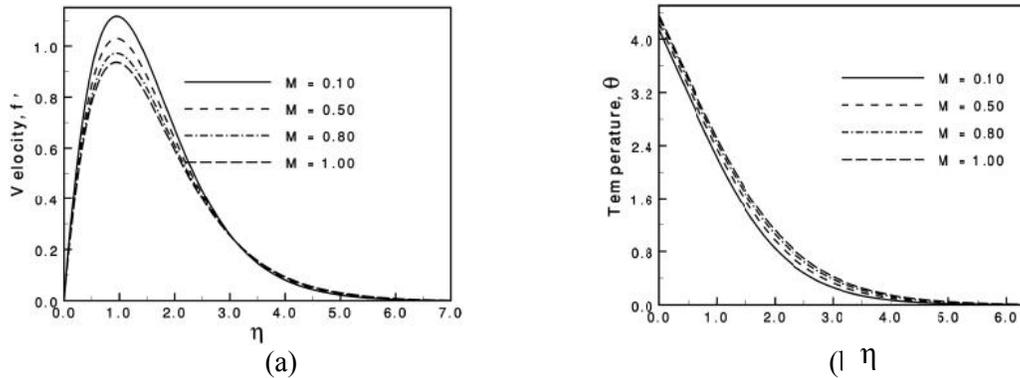
Fig. 2. (a) Variation of velocity profiles and (b) variation of temperature profiles against  $\eta$  for different  $M$  with  $n = 0.01$ ,  $Pr = 0.733$  and  $p = 0.25$ .
